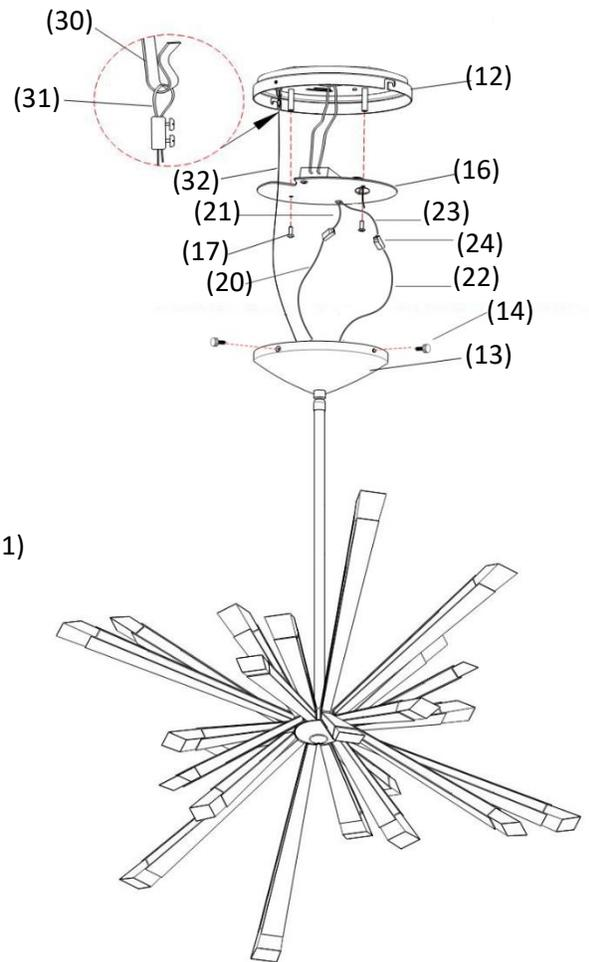
10. Insert the red+ fixture wire(20) into the quick connector(24) at the end of the red+ driver DC out wire(21); Insert the black- fixture wire(22) into the quick connector(24) at the end of the black- driver DC out wire(23). (As shown in Fig. 3)
